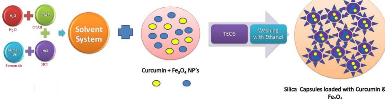
**Figure 5.** Schematic representation of loading of SiNPs with Curcumin and  $\text{Fe}_3\text{O}_4$ .
