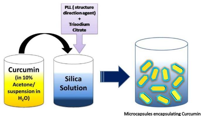
**Figure 6.** Synthesis of microcapsules encapsulating PLL-mediated self-assembled nanoparticles
