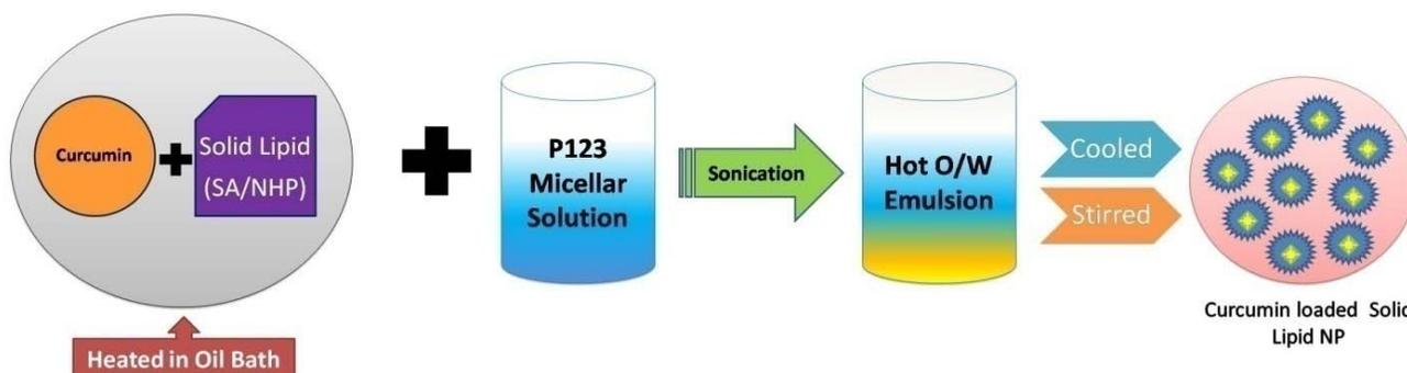
Figure 8. Synthesis of curcumin loaded nano matrix combining solid lipid nanoparticles and mesostructured silica.
