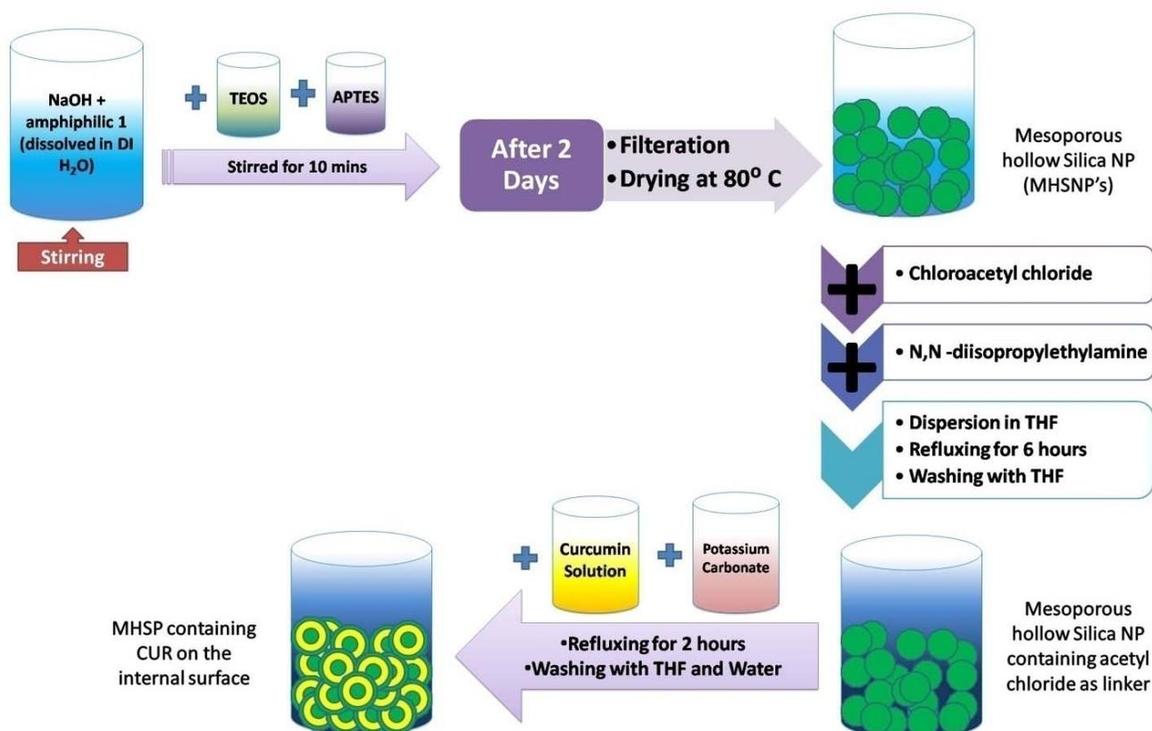
Figure 12. Synthesis and functionalization of C-MHSP using self-assembled alanine-based amphiphile as a template<sup>91</sup>
