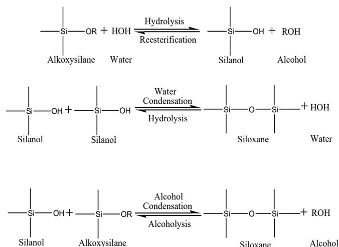
**Figure 3.** The hydrolysis of TEOS molecules forms silanol groups. The condensation/polymerization between the silanol groups or between silanol groups and ethoxy groups creates siloxane bridges (Si–O–Si) that form entire silica structure.
