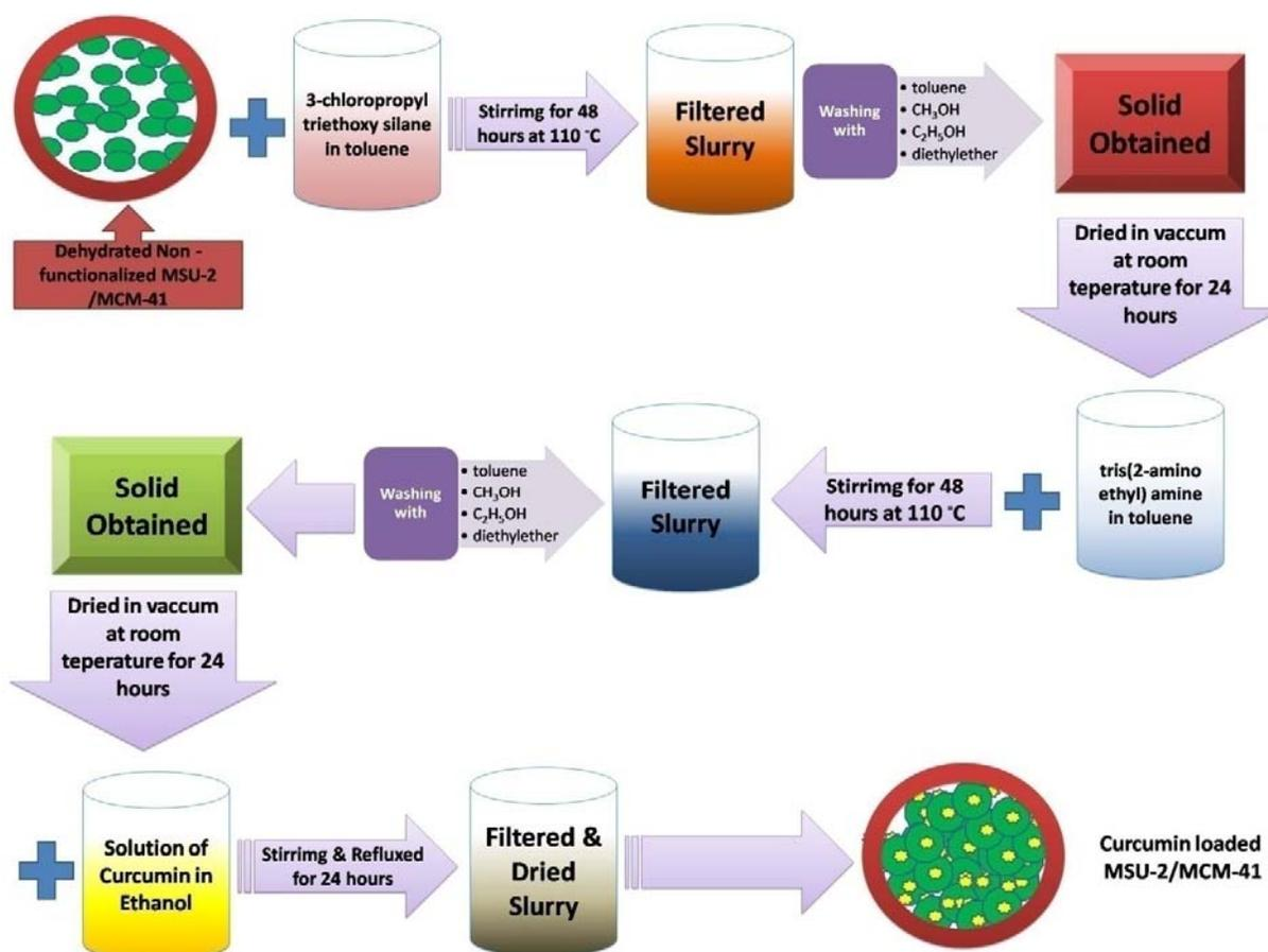
Figure 13. Synthesis of curcumin loaded MSU-2/MCM-41 by Bollu et al.<sup>103</sup>
