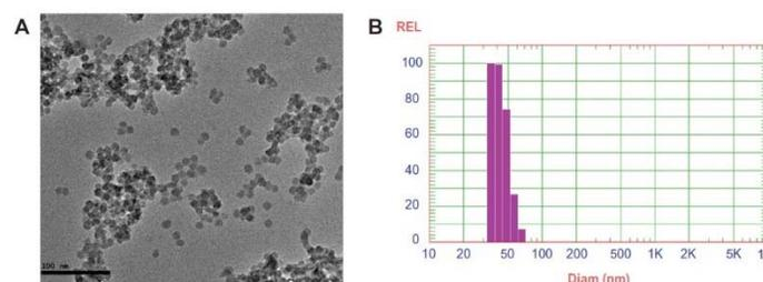
**Figure 15.** (A) Transmission electron microscopic image and (B) dynamic light scattering of silica nanoparticles coencapsulating gadolinium oxide and horseradish peroxidase. (Reproduced with permission from Ref. [167]. Copyright 2012 International Journal of Medicine)
