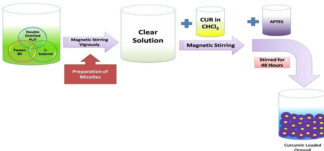
**Figure 10.** Synthesis of curcumin loaded organically modified silica (ORMOSIL) nanoparticles by Dinda et al.<sup>100</sup>
