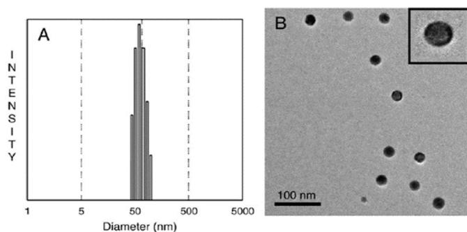
**Figure 14.** Representative (A) dynamic light scattering and (B) transmission electron microscopic images of the gadolinium oxide-doped and DNA-coated silica NPs. (Reproduced with permission from Ref. 166. Copyright 2011 Nanomedicine: Nanotechnology, Biology, and Medicine)
