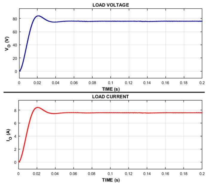
Figure 7. At  $(T_{ON} > 0.5 T_s)$  V-I characteristics through load
