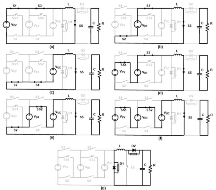
Figure 3. Working states of TIC operation in Buck-Boost mode
