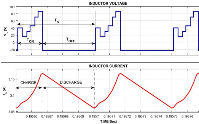
Figure 9. At ( $T_{ON} < 0.5T_s$ ) V-I characteristics through inductor (L)
