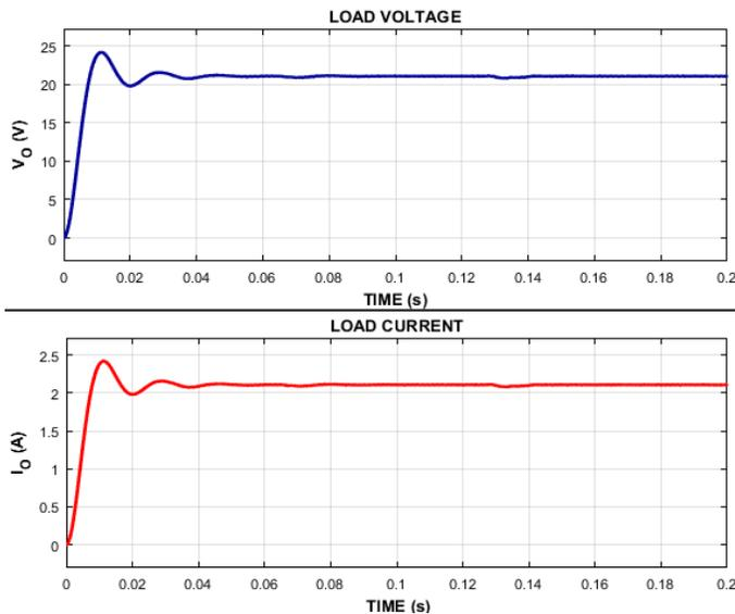
Figure 10. At ( $T_{ON} < 0.5T_s$ ) V-I characteristics through load
