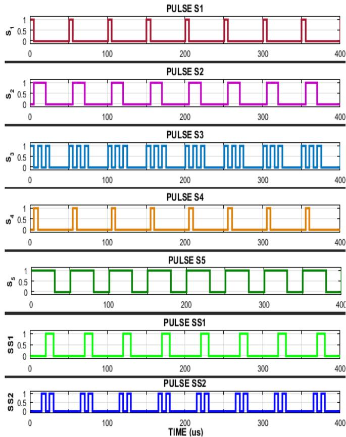
Figure 5. Applied Pulses at  $T_{ON} > 0.5T_s$
