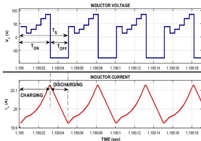
Figure 6. At  $(T_{ON} > 0.5 T_s)$  V-I characteristics through inductor (L)
