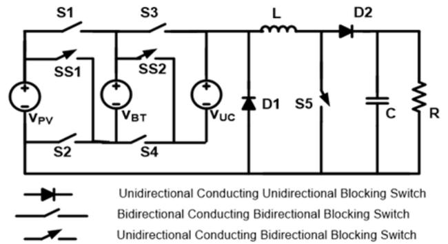
Figure 2. Equivalent Switch configuration of proposed TIC
