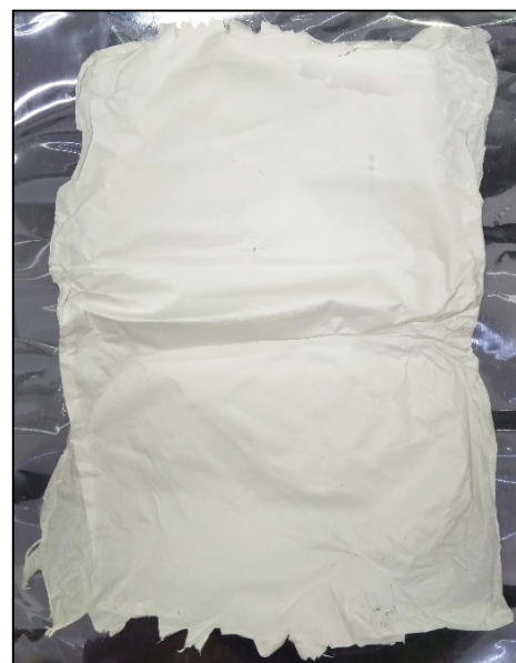
Figure 5: PVA/FG nanofiber sheet produced through electrospinning
