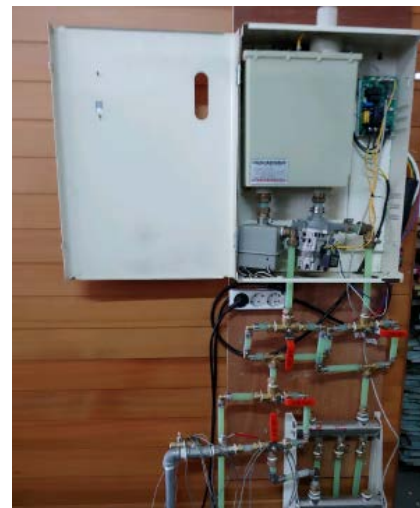
Figure 3. The experimental apparatus for natural convective radiative heat transfer cooling load of simple office for small factories
