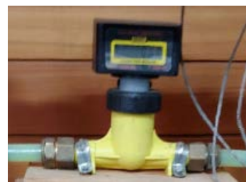
Figure 6. Flowmeter to measure the flow rate of cold water and temperature sensor to measure the temperature of cold water of simple office for small factories
