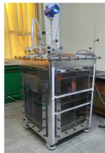
Figure 6. Test Apparatus showing the Water Tank with a Gas Collector inside
