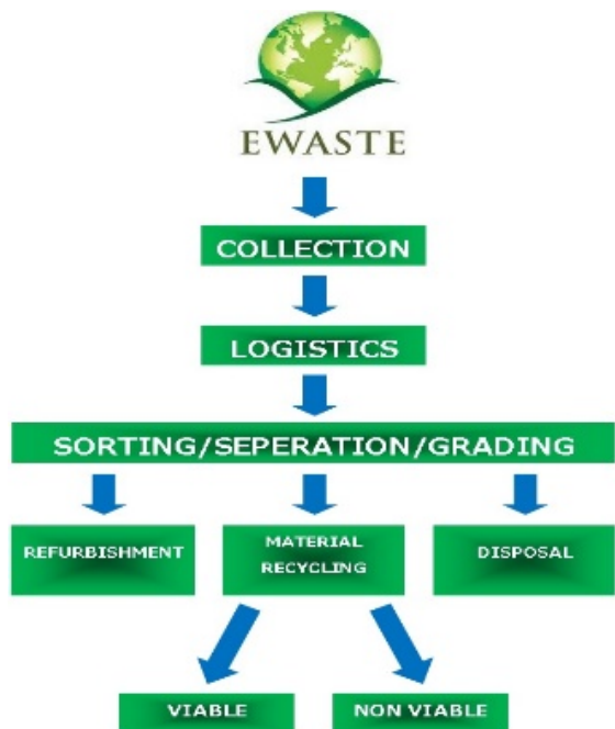
Figure 4. Flow chart of Recycling of electronic waste
