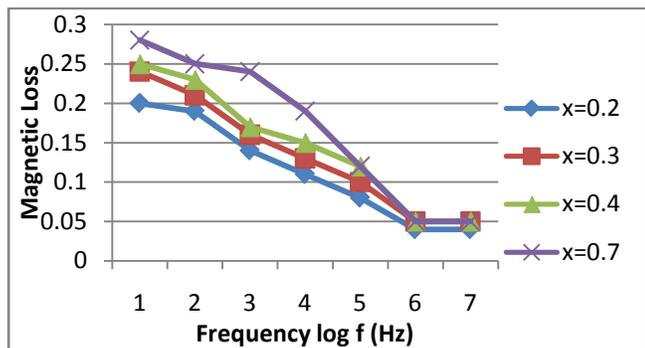
**Figure 3.** Variation of Magnetic Loss with Frequency of  $\text{Co}_x\text{Zn}_y\text{Fe}_2\text{O}_4$
